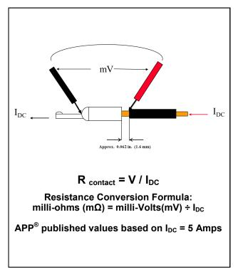
The included crimp performance and dimensional information are provided as a means to verify quality crimping of Anderson Power Products® contacts and is based on the use of tooling. The assembly of connector solutions with tooling assures that all crimp performance and fit specifications are met. Customers must regularly re-check electrical performance and dimensions of crimps to determine if APP® crimp tools require maintenance due to wear over time.
