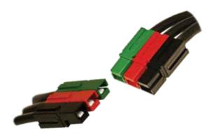
PP120 series Powerpole® housings are designed to accommodate up to 1/0 AWG (50 mm²) wires and handle high currents up to 240 amps. Reducing bushings allow PP120 to accept down to 8 AWG (10 mm²) wires. Multiple colors of stackable housings combine with low resistance flat wiping technology to offer powerful connection capability.
