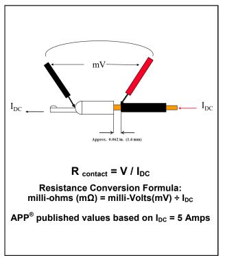
The included crimp performance and dimensional information are provided as a means to verify quality crimping of Anderson Power Products® contacts and is based on the use of tooling. The assembly of connector solutions with tooling assures that all crimp performance and fit specifications are met. Customers must regularly re-check electrical performance and dimensions of crimps to determine if crimp tools require maintenance due to wear over time.
