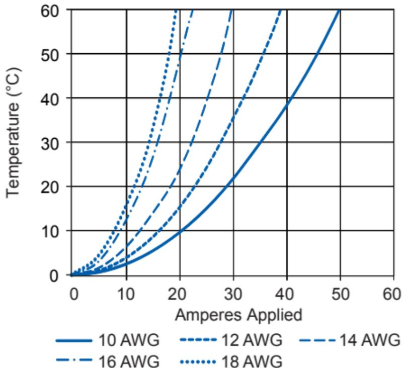
NOTE: Temperature rise chart is based on a 25°C ambient temperature.
