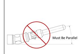
The original geometries of the contact should be maintained after crimping (except in the crimp indent area).
