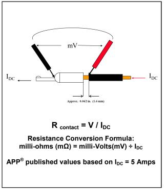
The included crimp performance and dimensional information are provided as a means to verify quality crimping of Anderson Power Products® (APP®) contacts and is based on the use of APP® tooling. The assembly of connector solutions with APP® tooling assures that all crimp performance and fit specifications are met. Customers must regularly re-check electrical performance and dimensions of crimps to determine if APP® crimp tools require maintenance due to wear over time.
