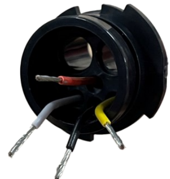
Figure 8: Auxiliary wires fed through main plug housing with bottom three wires bent out of way
