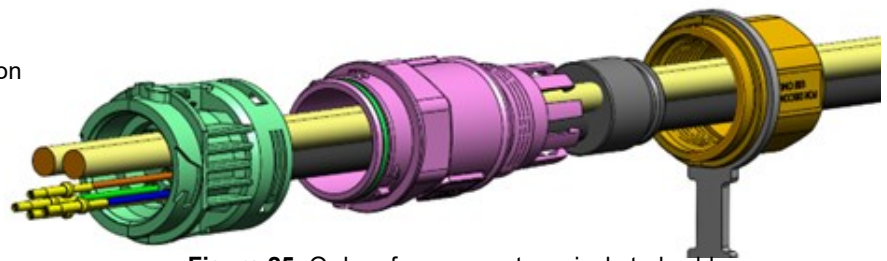
Figure 25: Order of components on jacketed cable
