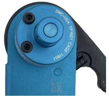
TM0001 with Locator Installed
