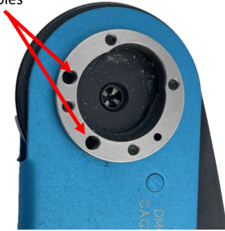
Locator Installation Area
